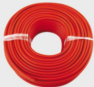
EN559 (8mm LP Gas Hose Class 2 Max W.P 10 Bar Propane/Butane BS3212/EN1763)
